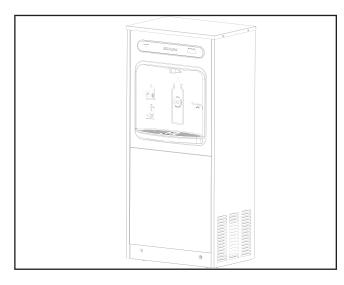
3. Remove the lower front panel by removing the two hex screws on the cooler unit using a 5/16" socket or nut driver.
