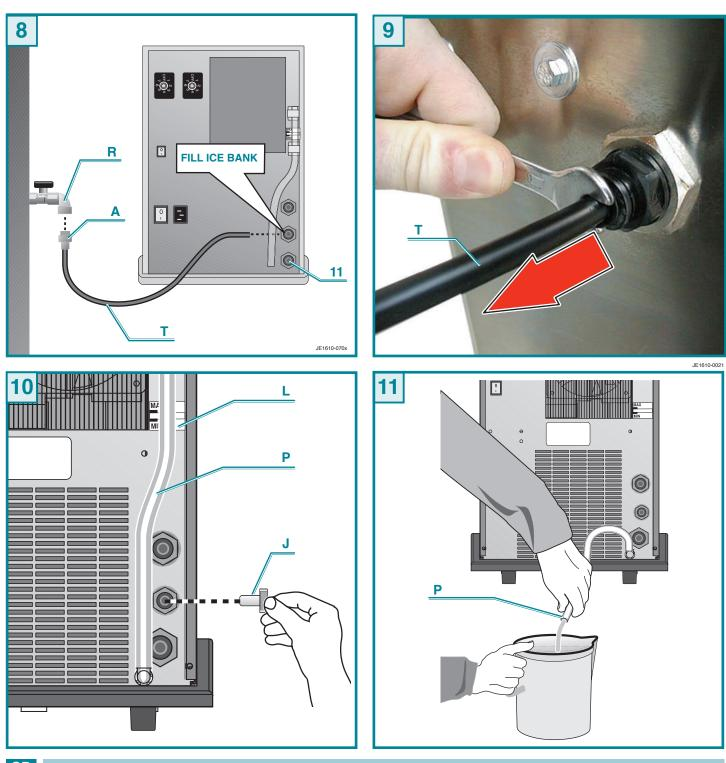
Connection to the water mains is done using the  ${\bf T}$  tube provided (8 mm diameter) and by terminal A (3/8M) for 8 mm pipe.
