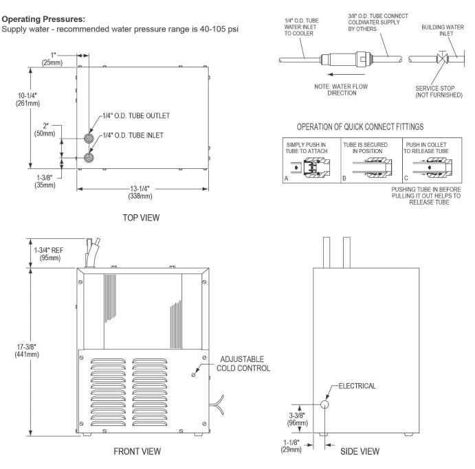
NOTE: When mounting unit in an open area, to ensure proper ventilation, maintain a 4" (102mm) clearance from cabinet louvers on each side of chiller. When mounting unit in a cavity or behind a wall, maintain minimum space of 4" (102mm) on each side, 4" (102mm) on the top and a depth of 12" (305mm).
