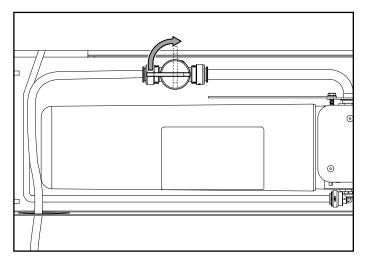
3. Activate the water dispenser using a water bottle to relieve pressure in the water line.
